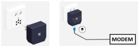
When the modem and the telephone sets are installed far from the NTP, appropriate cables can be connected on the blue (for VDSL) and green (for telephony) screw terminals inside the NTP (the cover of the NTP can be unscrewed). The VDSL blue terminals are only active when the splitter is plugged into the NTP.
